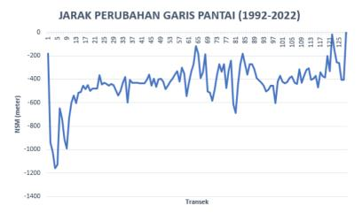
The rate of change of the North Coast of Bengkalis Island, Prov. Riau is obtained by using the value of EPR (End Point Rate). End Point Rate is defined as the calculation of the rate of change of the coastline by dividing the distance between the longest coastline and the current coastline by the time. The formula used is as follows;
