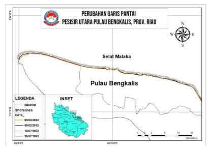
The results of the analysis of shoreline changes are then used to make predictions (forecasts) using ArcGIS 10.5 software using the Digital Shoreline Analysis System (DSAS) method. The results of the coastline prediction obtained are shown in Figure 2. Based on the map, it is known that the prediction of the coastline in the next 20 years the north coast of Bengkalis Island will experience abrasion. The highest abrasion occurs on the west coast of the island of Bengkalis.
